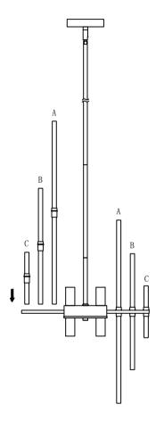
1. Put the glass bars A, B, C into the slot, and then twist the bulb to power on.
